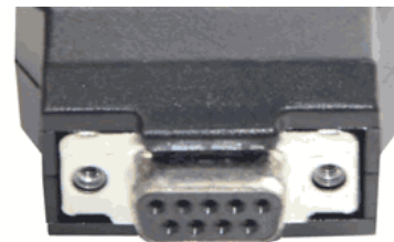
Example Female RS-232 Connection
