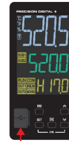
Mini-USB Port Location for PD520 and PD530: Front Panel, Lower Left
