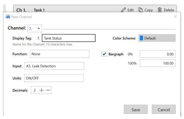
You will notice that the "Units" default to "ON/OFF". The reason this happens is because since the "Function" is none, the ConsoliDator+ knows that we are trying to setup an "Annunciator Screen" and they gives us the typically used, "ON/OFF" units.
