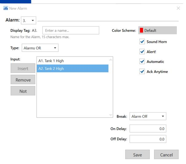
There are a couple things to notice here. For starters, you will notice that we are not entering any setpoints or reset points. That is because that was done at the "Single Source" alarm level. Remember, this "Alarm" is simply a way for us to combine our "Conditional Statements" to perform complex control!
