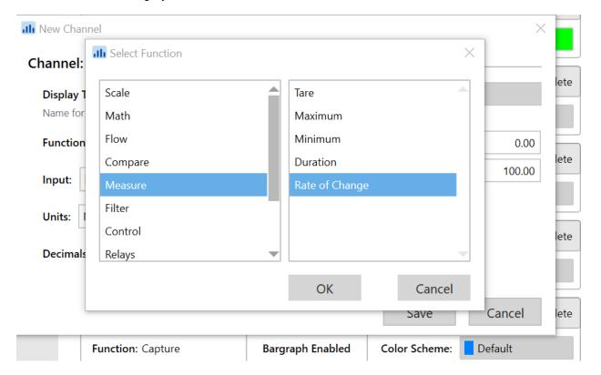
Once you select your function, you choose which input this channel will monitor the rate of change. So, in this example, we want our 1,000 gallon tank channel to be the "Input" here. Select that channel as the input.
