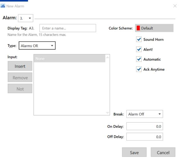
Once you have selected the correct "Type", you can now start "Inserting" the other alarms that you would like to have on this alarm. In this example, we want the high alarms for our two tanks to be on this alarm.
