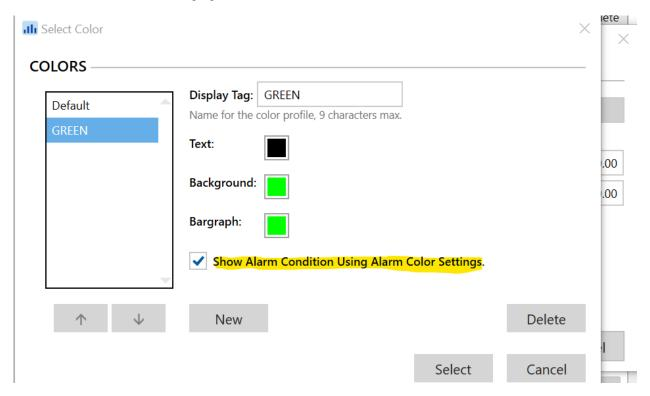
Without that box checked, when our leak detection alarm triggers, the color of this channel will NOT change. Yes, the message will change as it should, but to really take advantage of the ConsoliDator+, having the channels change color on alarm is a really nice thing to add!
