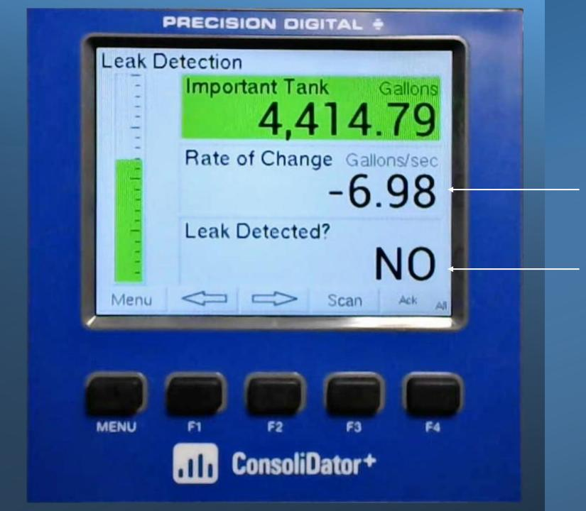
When the tank is emptying, the reading will be a negative number. It will be positive if the tank is being filled
