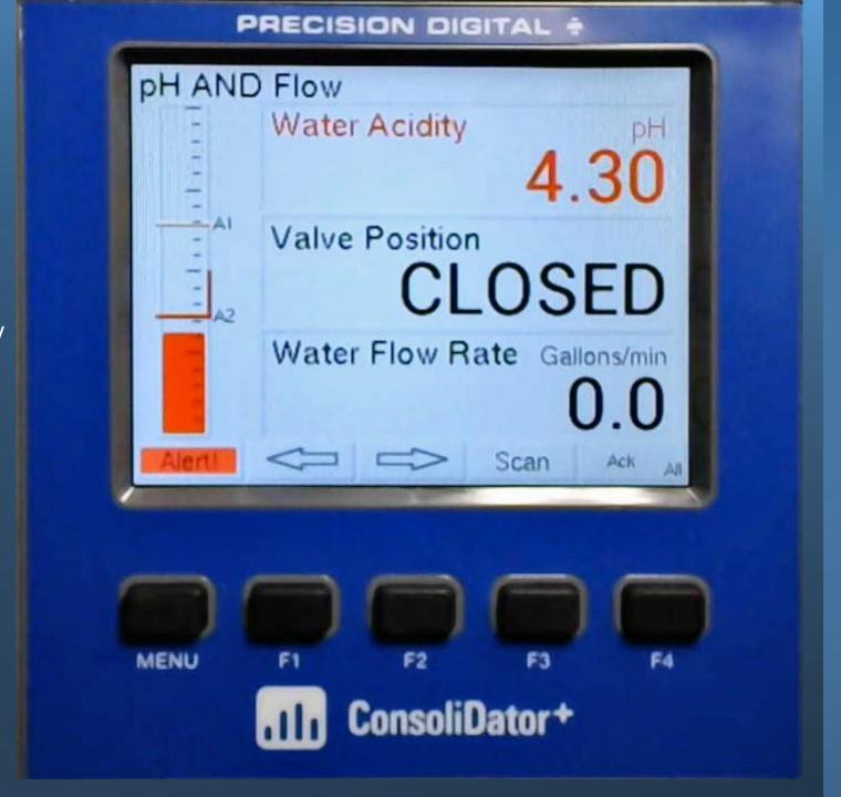
So, regardless of in which direction our pH falls, if it is not as close to 7 (neutral) as possible, then the ConsoliDator+ will force the valve closed, and therefore cutting off the flow rate!
