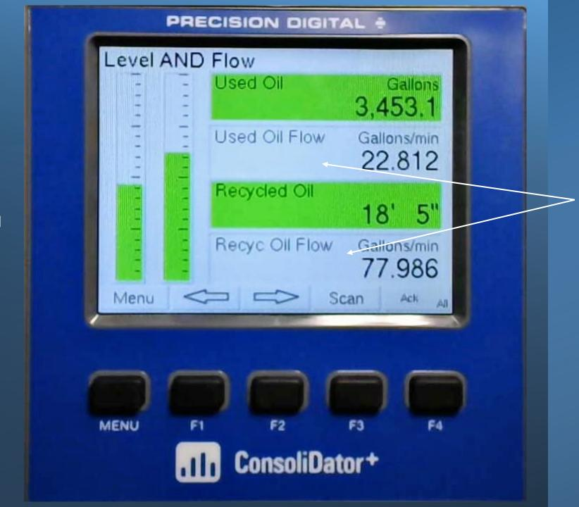
However, we are also monitoring the flow rate of the oil BETWEEN these two tanks at the same time, on the same screen!
