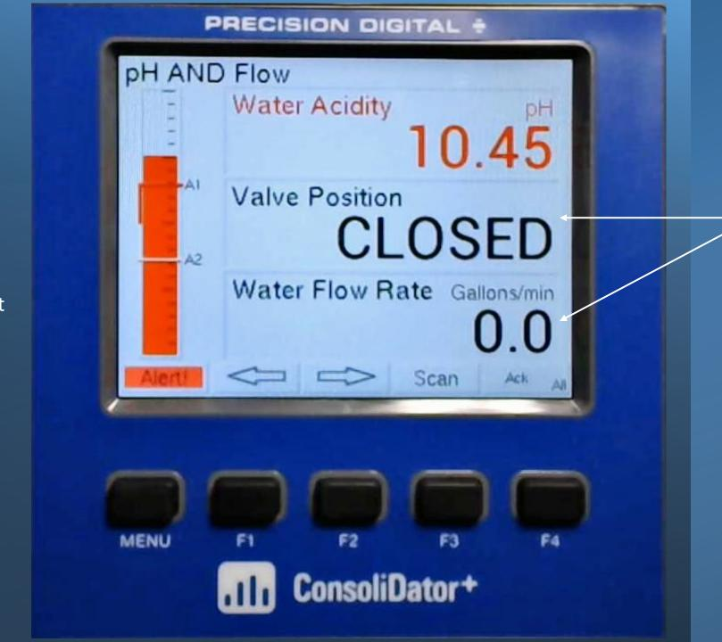
Since our water is becoming more acidic, the valve will close so that the water cannot flow out into the public water supply.
