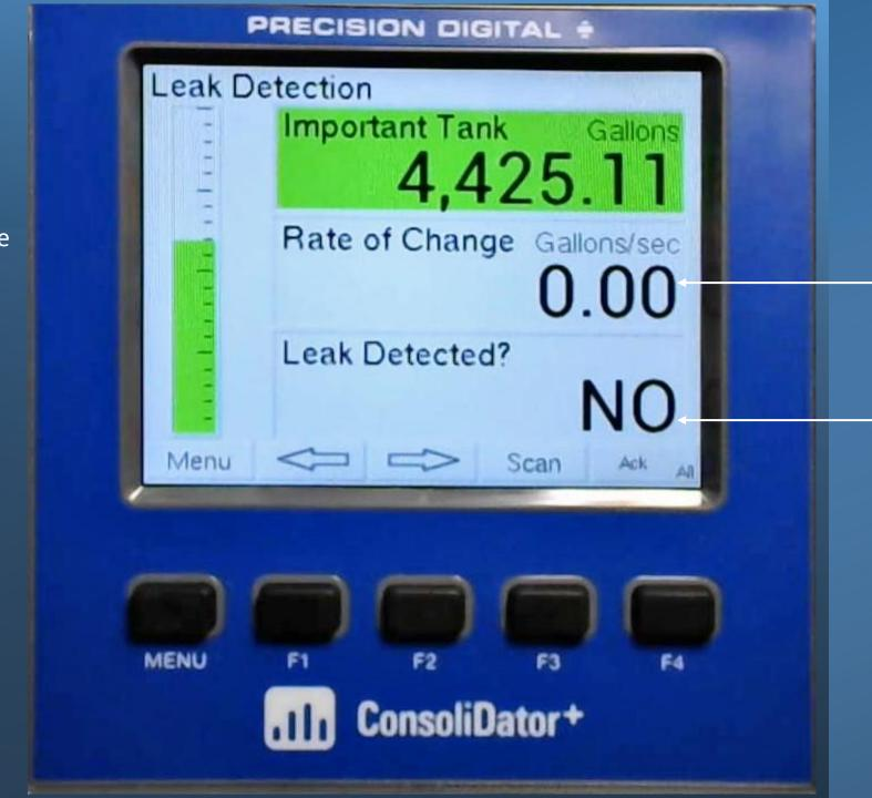
The "Rate of Change" channel is quite literally monitoring the rate of change in level in this tank.
