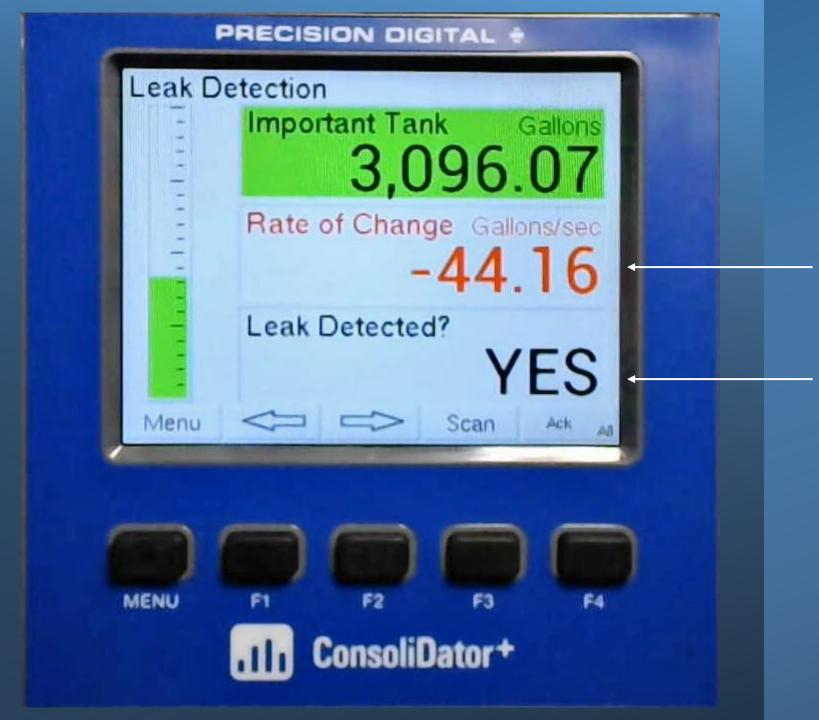
When the "Rate of Change" exceeds a specified threshold, the channel goes into alarm
