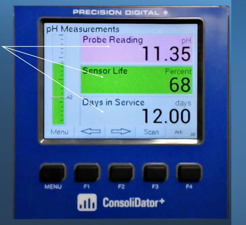
NOTE: The "Sensor Life" and "Days in Service" is going to be read using the Modbus protocol.
