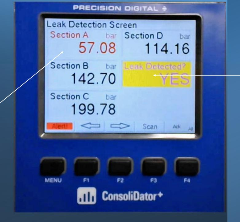
Now that Section A is in alarm, our "Lead Detected?" alarm channel now says, "YES, there is a leak" and the color is now an extremely ugly combination of YELLOW and PINK.
