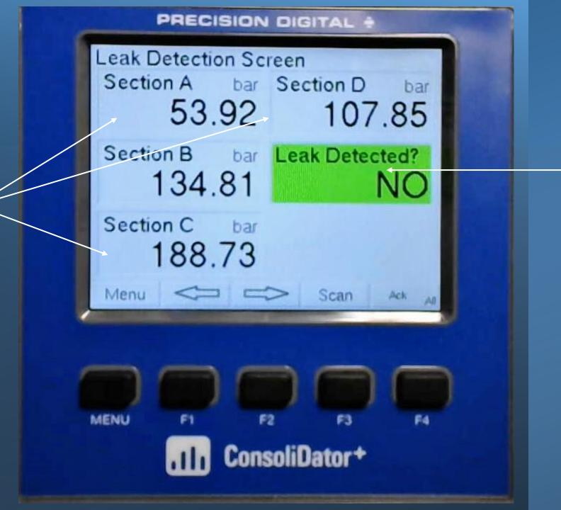
to be operating normally, so our "Lead Detected?" alarm channel is GREEN, and it's letting us know that there are no leaks present.
