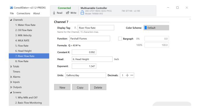
Above is a screen shot of what it looks like when you setup an open channel flow channel using the <u>ConsoliDator+ Configuration Software</u>. You will notice my "Function" is Parshall Flumes and that will automatically generate the "Formula" you can see below.
