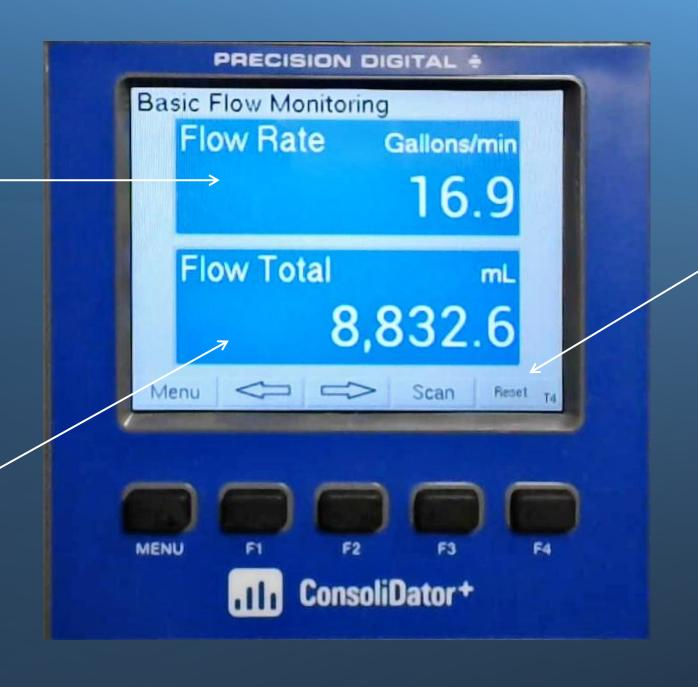
We can use a "Soft Key" to reset the total shown on the screen.
