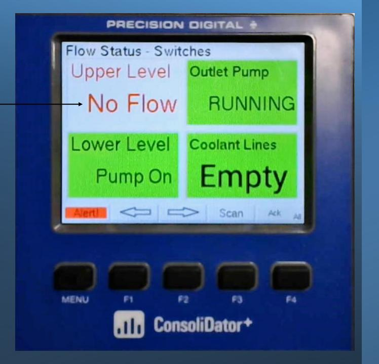
You cannot see it on the slide, but the "Upper Level" channel has not only turned red, but it is flashing to catch the operator's attention.
