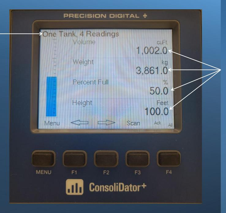
In this example, we only have four readings, but you COULD actually make 160 completely unique readings based off just ONE process signal
