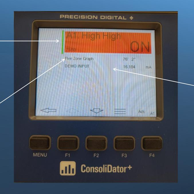
Lastly, it can show you exactly which INPUT is tied to the channel that is in alarm.
