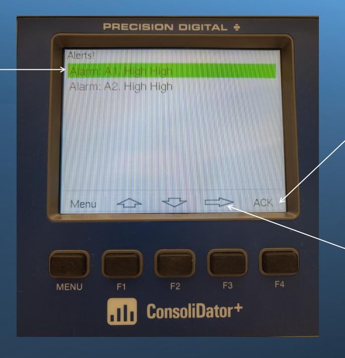
By using the "Up" and "Down" arrow keys, you can highlight a specific alarm, and choose to acknowledge the alarm right from this screen!
