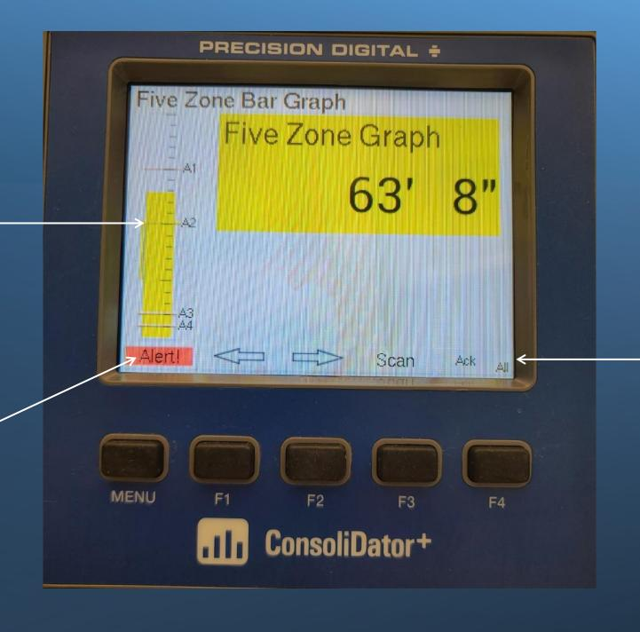
A "soft key" can be programmed on any screen to allow an operator to acknowledge an alarm which is especially useful if they have the alarm tied to an audible alarm that needs to be turned off while they address the issue.
