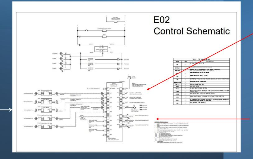
Relays (10 amps) being used for high level alarm AND pump control...
