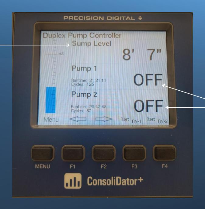
The ConsoliDator+ can show you pump status and can also keep track of pump cycles and runtime! As the level of the sump rises, and approaches our "A5" alarm marker, we want to pump out some of the material.
