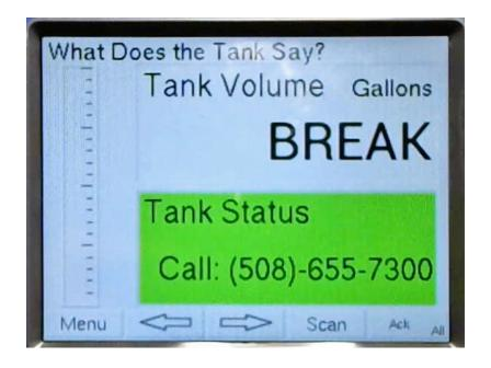
**PROBLEM:** Your customer monitors the level of their wet well with two separate technologies. Their primary sensor is a submersible pressure transducer, and the other is an ultrasonic sensor suspended from the top. However, sometimes the submersible transducer stops working, or the wires get cut, and then they don't have an easy way to maintain their level readings on the same device!!
