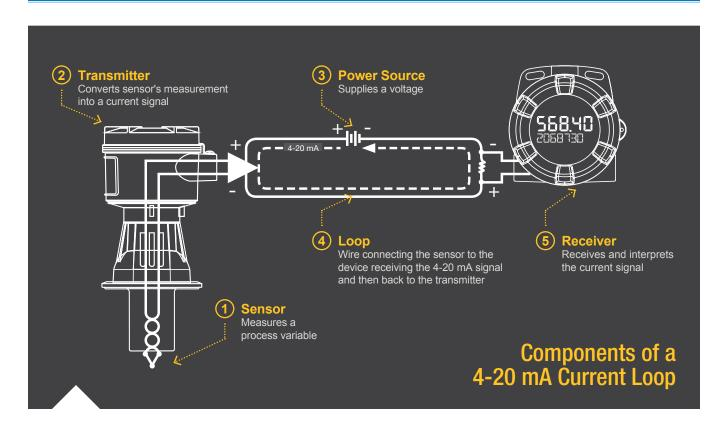
height of a fifty foot tank, the transmitter would need to translate zero feet as the tank being empty and then transmit a four milliamp signal. Conversely, it would translate fifty feet as the tank being full and would then transmit a twenty milliamp signal. If the tank were half full the transmitter would signal at the halfway point, or twelve milliamps.
