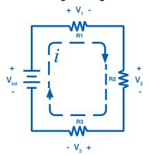
Consider the simple DC circuit above, consisting of a power supply and three loads. A current loop requires voltage to drive the current. This is provided by the power
