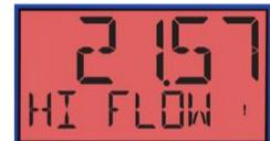
Meter in alarm condition. Display turns red, flashes and shows HI FLOW alarm message.
