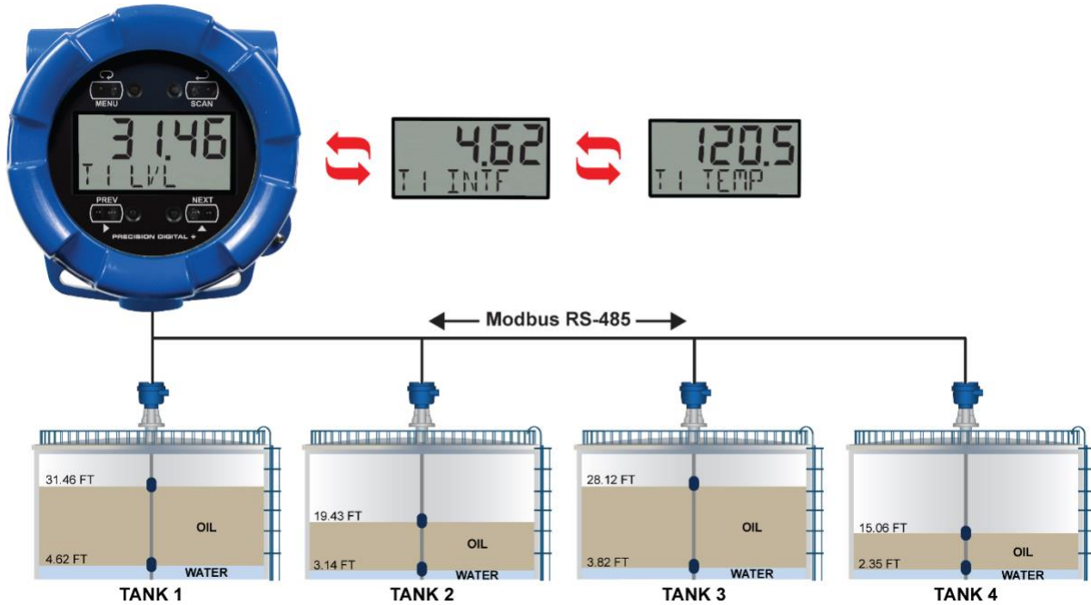
Example 1 Level Transmitter Setup, Register Numbers, & Process Variables
