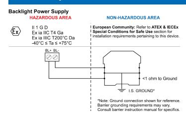
Backlight Power Supply Connection Entity Parameters: Ui = 30 V, Ii = 175 mA, Pi = 1 W, Ci = 0, Li = 0
