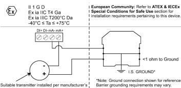
mA Input Connection Entity Parameters: Ui = 30 V, Ii = 175 mA, Pi = 1 W, Ci = 0, Li = 0
