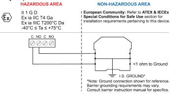
Relay Output Connection Entity Parameters: Ui = 30 V, Ii = 1.0 A, Pi = 1 W, Ci = 0.013  $\mu$ F, Li = 0 Uo = 11.55 V, Io = 0.001, A Po = 0.012 W
